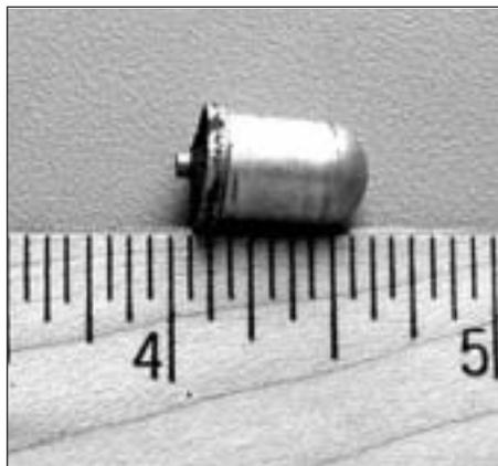
Not all vehicles contain mercury lighting switches. The number of mercury light switches in a vehicle is estimated to be between 0.54 switches and 0.8 switches per vehicle (2 & 3). The average amount of mercury in a switch is 1.2 grams (3).
